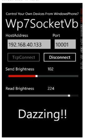
Controlling the brightness of the LED with the upper slide bar and showing under slide bar read brightness. Thank you for reading.
