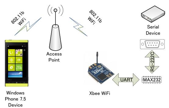
WindowsPhone7.5 device connects to XBee WiFi over TCP socket.
